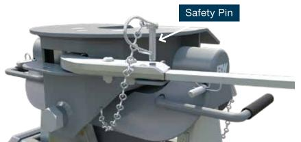
Use the safety pin to lock the handle in the open position and when you are sure that the landing gear will support the trailer, move the truck forward to release the jaws from the kingpin.
