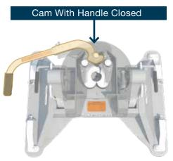
We designed our jaws and handle to work with a cam mechanism. When the handle is pinned closed, the cam keeps the jaws from opening.
