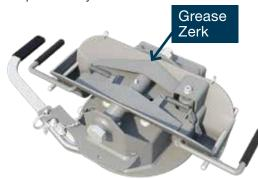
Spread a thin layer of multi-purpose grease around the inside surface of the jaws where they grasp the kingpin. You may also want to apply some grease to the kingpin on your trailer.
