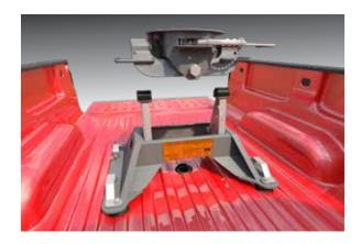
**2.** Remove the latch pins from each of the handles.
