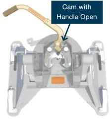
When the handle is open the cam allows the jaws to open, even if you are in a bind because of unlevel ground. If the handle is open, you may go ahead and drive out of the jaws. They will open as you pull away.
